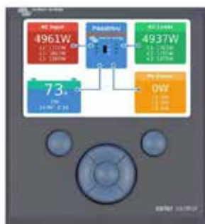
Color Control GX, showing a PV application
