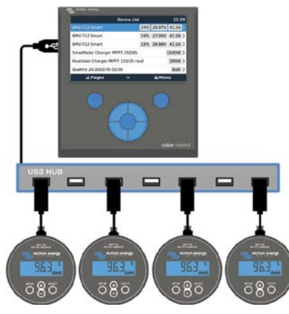
A maximum of four BMVs can be connected directly to a Color Control GX. Even more BMVs can be connected to a USB Hub for central monitoring.
