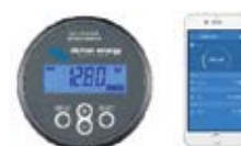
BMV-712 Smart Battery Monitor The BMV Battery Monitor features an advanced microprocessor control system combined with high resolution measuring systems for battery voltage and charge/discharge current. Besides this, the software includes complex calculation algorithms, like Peukert's formula, to exactly determine the state of charge of the battery. The BMV selectively displays battery voltage, current, consumed Ah or time to go. The monitor also stores a host of data regarding performance and use of the battery.
